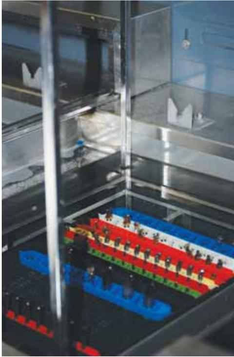
Hardcoating parts in carrier.
