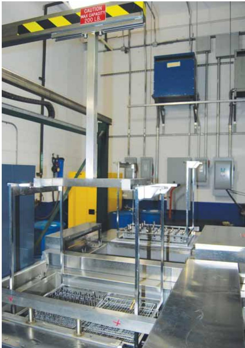
Multiple loads and recipes move simultaneously through the Miraclean ultrasonic cleaning line, which has tripled precision cleaning throughput at HTL.
