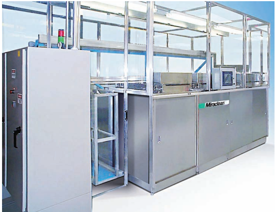
Custom medical cleaning line with ventilated enclosure.
